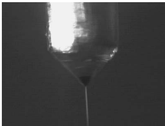
Fig. 2. Optical micrograph of a stable Taylor cone mode of a 10% (w/w) paracetamol solution in ethanol. The electrohydrodynamic conditions were established at a flow rate of 1.2 ml/h, an applied DC voltage of 3.8 kV, and a 5-cm separation distance between capillary and grounded reference.
